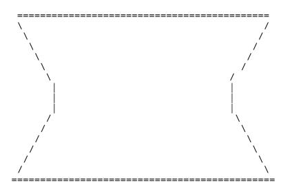
This geometry is the natural state of affairs with linear scan waveforms if there were no correction. Normally, a signal from the vertical deflection that looks something like a rectified sinewave is used to modify width based on vertical position. There is usually a control to adjust the magnitude of this signal and also often, its phase. It would seem that this circuit has ceased to function.
